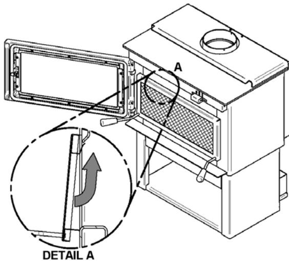
Lean the upper part of the fire screen against the top door opening making sure to insert the top fire screen brackets behind the primary air deflector as in (Detail A).
