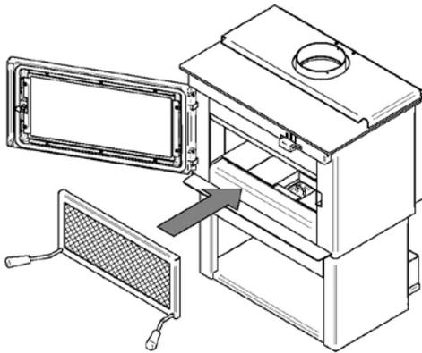
Hold the fire screen by the two handles and bring it close to the door opening.
