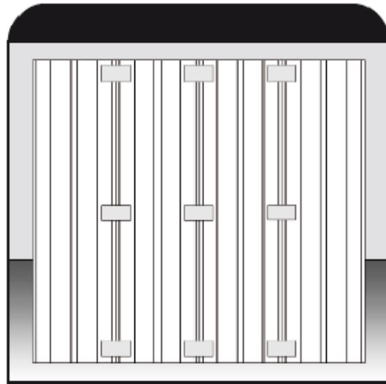
■ Evenly space 3 pieces of aluminum tape along the joint. Repeat at each joint to form a single unit.
