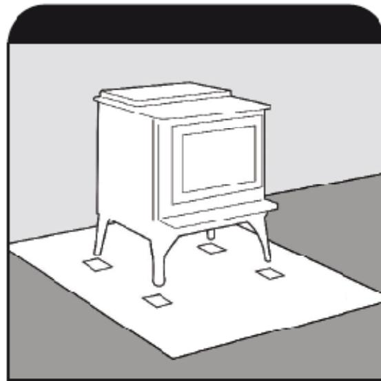
■ For stoves with legs, place a Load Spreading disk (included) underneath each leg to prevent pressure cracks.
