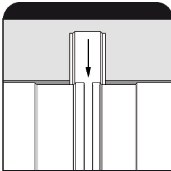
■ Wearing gloves, insert a locking strip under the metal edges of two panels where they meet. Slide the strip down to the floor. Repeat at each joint.
