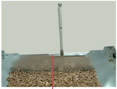
Using vise grips squeeze the cable protector and the hopper switch bracket as tight as possible against the sides of the hopper.
