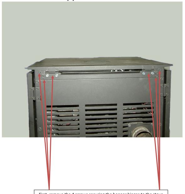
First, remove the 4 screws securing the hopper hinges to the stove and then the 4 screws securing the hopper lid bumper support.
