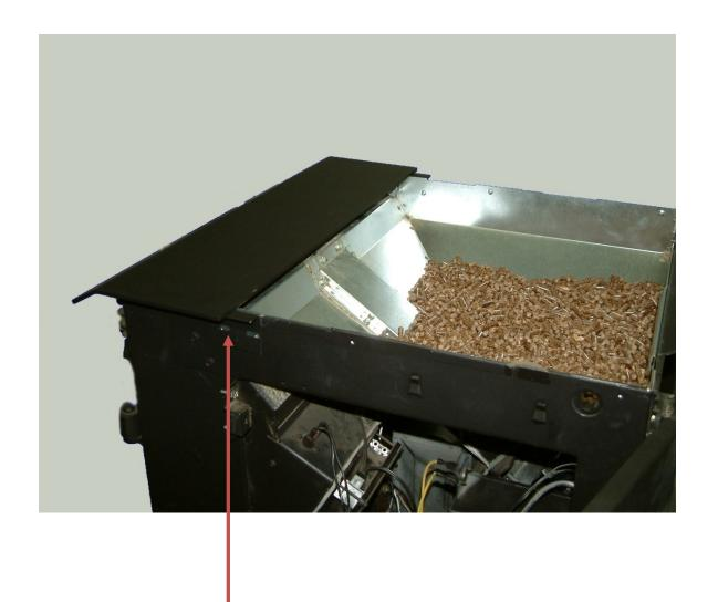
Secure the new top using the front screw only. The other hole will be used later to secure the hopper extension.
