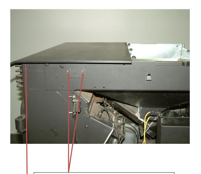
Open the decorative panel on both sides and remove the two screws securing the top to the stove.
