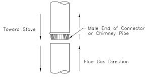
FIGURE 2.3 (A) Connecting Sections
