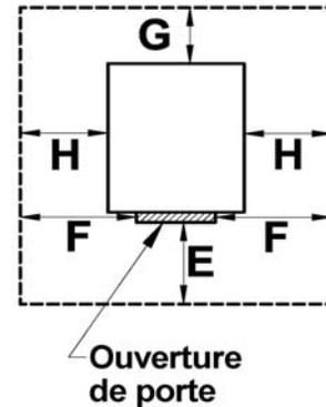
**AVERTISSEMENT: LE POÊLE DOIT ÊTRE PLACÉ SUR UNE SURFACE INCOMBUSTIBLE CONTINUE TELLE QUE DE LA CÉRAMIQUE\*, UN PANNEAU DE BÉTON, DE LA BRIQUE, UN PANNEAU D'AGGLOMÉRÉ INCOMBUSTIBLE OU TOUT AUTRE MATÉRIEL ÉQUIVALENT, APPROUVÉ COMME PROTECTION DE PLANCHER.**
