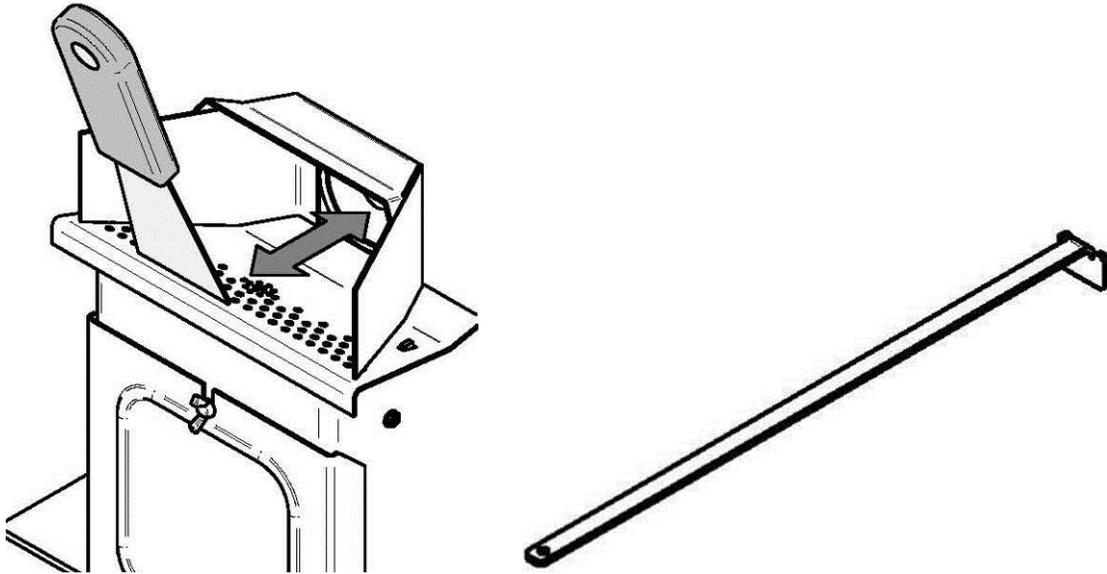
2. The burn pot (**A**) simply sits onto the air intake channel. You must lift to remove it from the stove. Two small pins guide the burn pot in place. Make sure that the burn pot is well in place before turning on the stove (as shown in the diagram).
