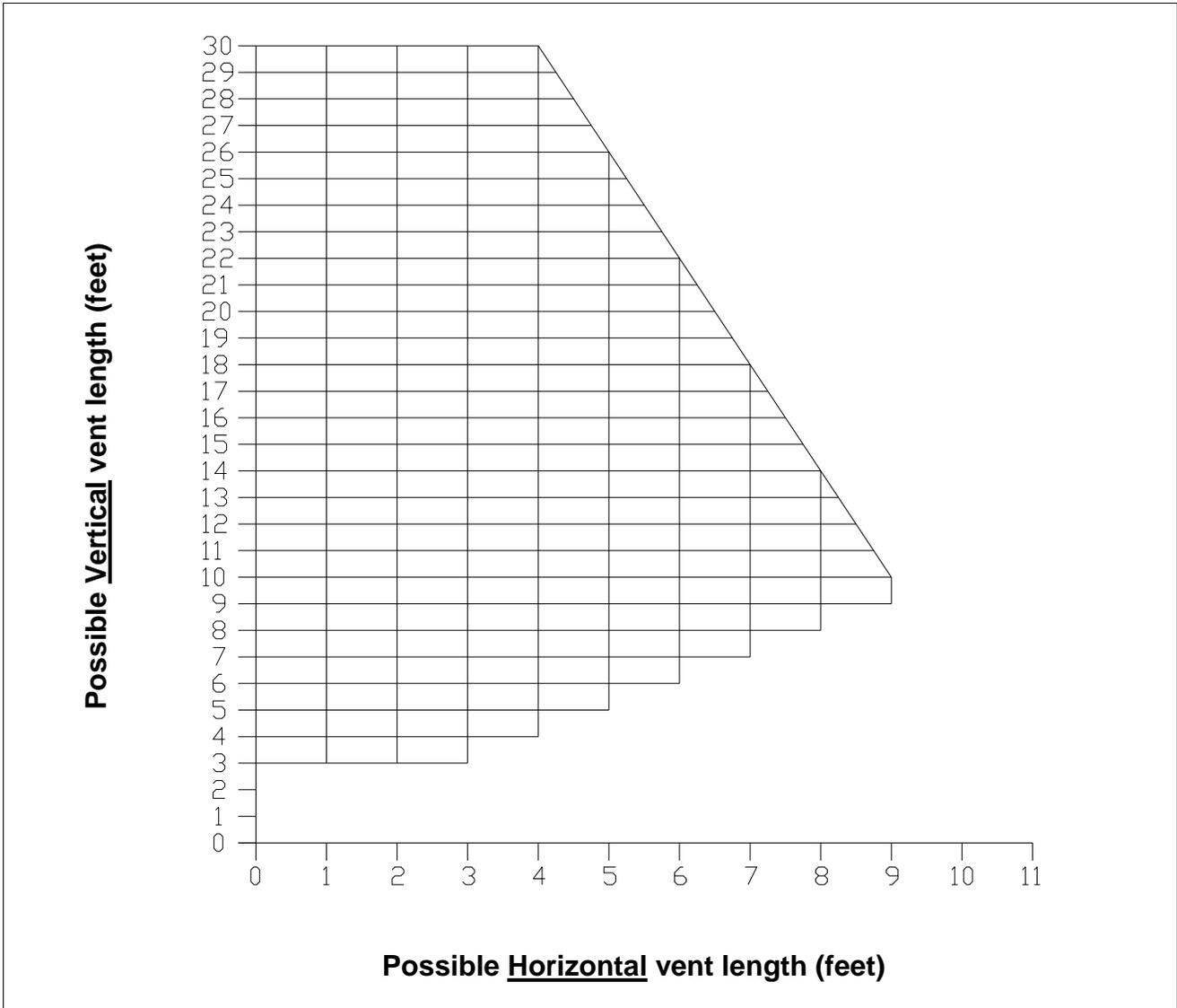
For example, let's imagine an installation consisting of a horizontal vent coming out at the back of the stove on a total distance of 8 feet. This horizontal run is followed by a tee and a 6-foot vertical rise. This type of installation is not acceptable. As you can see, the vent termination is clearly outside the allowed configuration zone on the chart because the venting system proposed **does not have at least one foot of vertical rise for each foot of horizontal run.**
