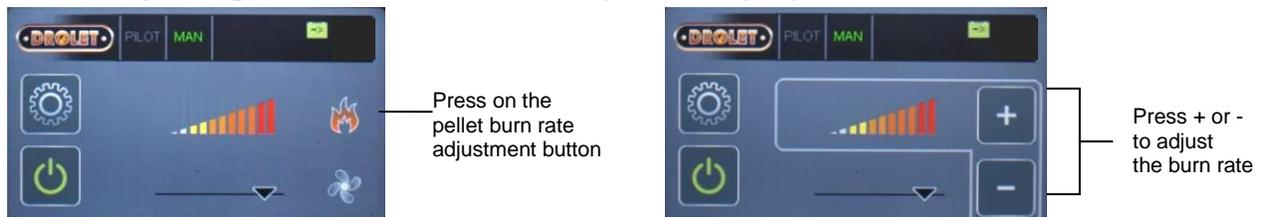
The stove's input range goes from 10,000 BTU/h to 45,000 BTU/h. To change combustion level, select the flame icon
