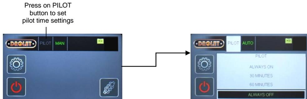
**Note:** Pilot feed rate is lower than the minimum combustion level feed rate.
