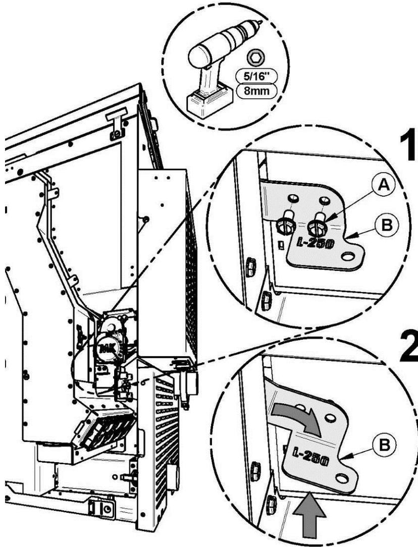
Remove the faulty thermal switch. Replace new thermal switch **(D)** underneath the bracket **(B)** by means of 2 screws **(C)**.
