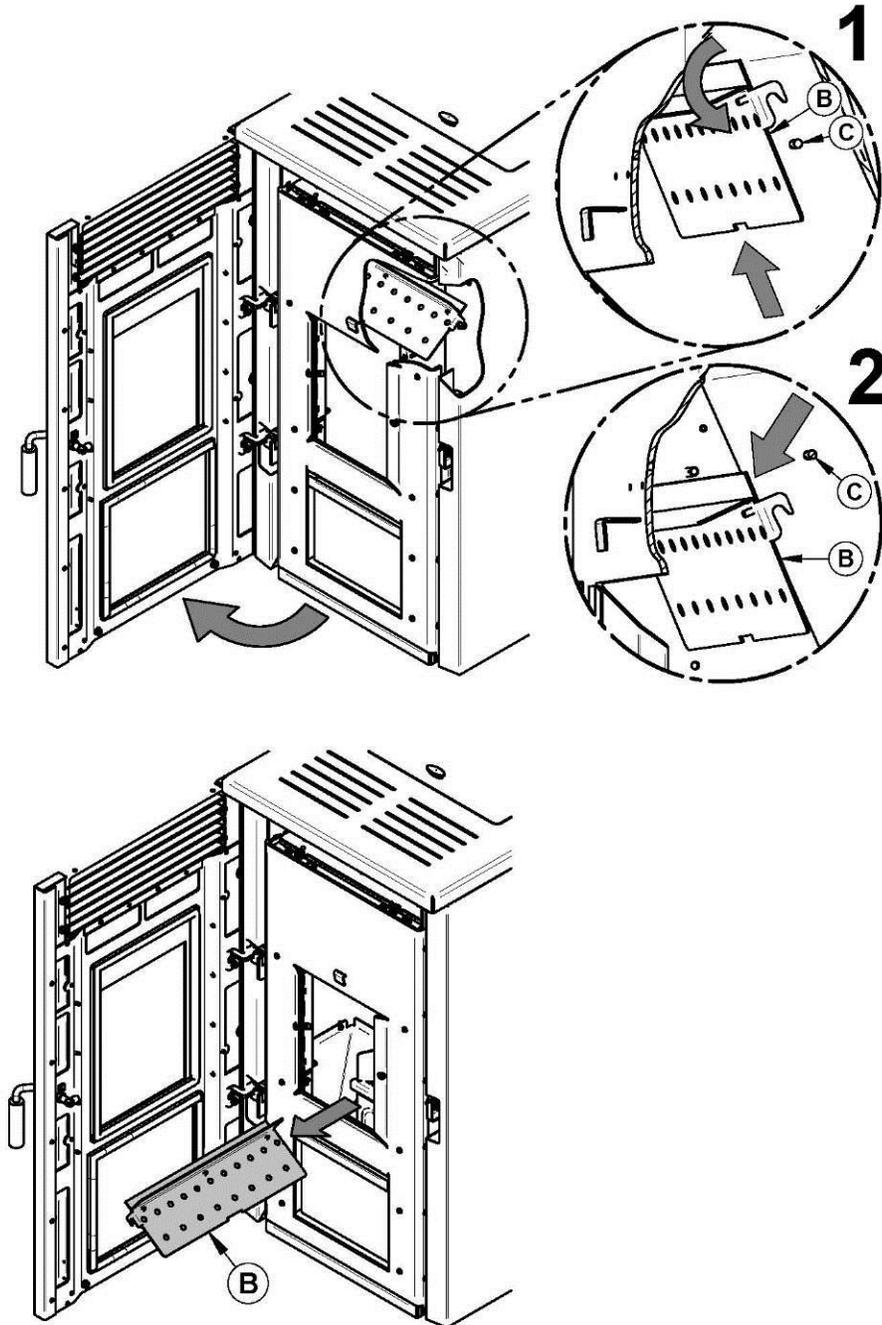
**IT IS HIGHLY RECOMMENDED TO CLEAN THE EXHAUST CHANNEL (SEE SECTION 8.1.3: EXHAUST CHANNEL AND EXHAUST BLOWER MAINTENANCE) IMMEDIATELY AFTER CLEANING THE HEAT EXCHANGER.**
