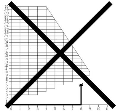
Instead, if the installation consisted of a horizontal vent coming out at the back of the stove on a total distance of 4 feet, followed by a tee and a 6-foot vertical rise, it would be acceptable. The termination is within the allowable configuration zone on the chart since it would have at least one foot of vertical rise for each foot of horizontal run. Furthermore, the total vertical rise is at least 3-feet high.
