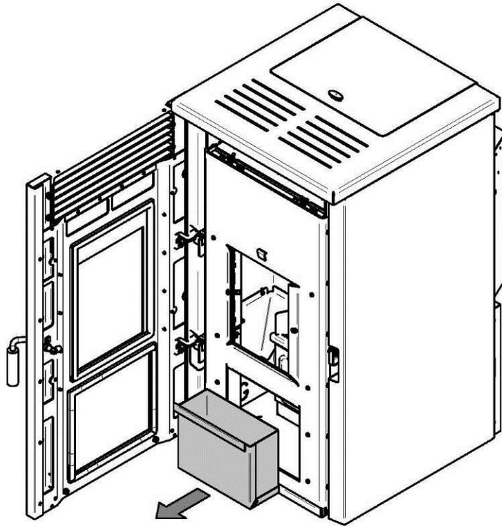
4. Unscrew the wing nut (C) to open the clean out trap (B). Vacuum the combustion residues.
