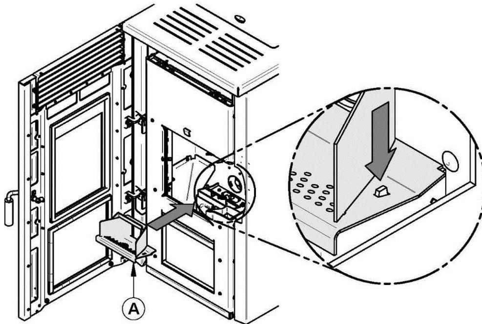
3. If necessary, clean the air intake channel. To reach the air intake channel clean out trap, open the door and remove the ash drawer.
