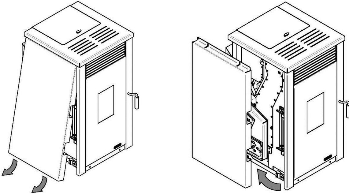
Using a Philips or Robertson screwdriver, remove both clean-out traps **(E)** and **(F)** by unlocking them. Push the screw and give it a counter-clockwise quarter turn. Clean the pressure sensor located on the rear access panel.
