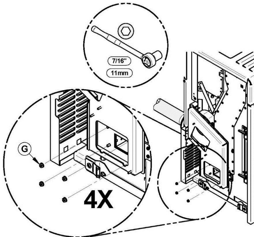
Remove the duct assembly (H).
